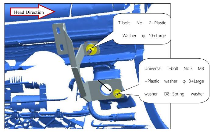
3) Installation of middle brackets (symmetrical)
