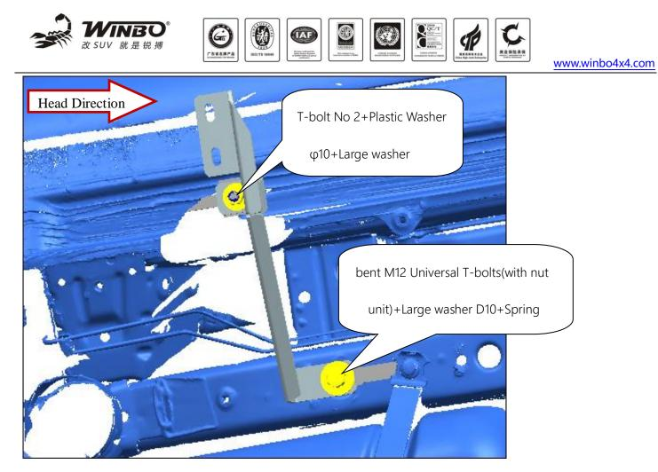
Step 4 : Installation of Running board
