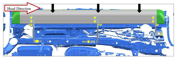
Step 5 : Recover the chassis's plate back to the car and mark those places with pencil in order to cut with free space to contain running board.
