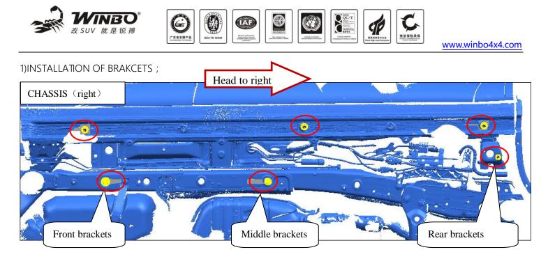
2) Installation of front brackets (symmetrical)
